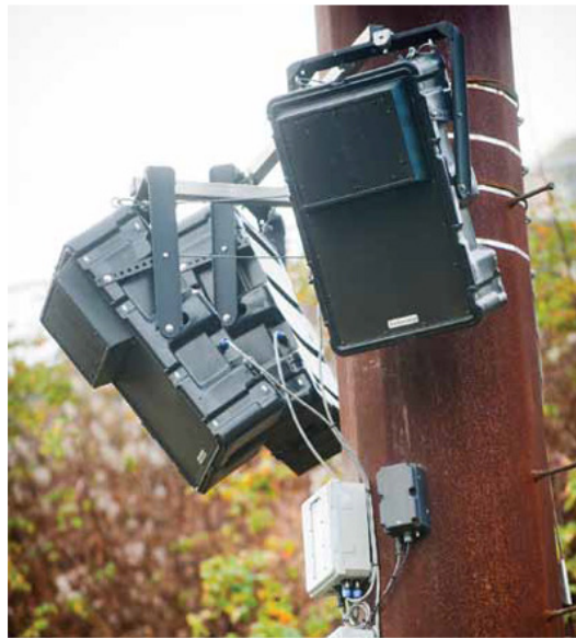
Technomad's Berlin loudspeakers and PowerChiton amps enable designers to deliver multichannel audio to outdoor audio projects, with multi-decade lifespans.
